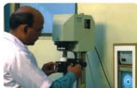
Laser Interferometer for optics inspection
